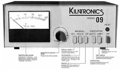
Refer to the front panel of your Temperature/Rate Controller as you read through the following explanation of what each front panel feature is and does. Don't be afraid to push the buttons and turn the knob. You won't break anything.
