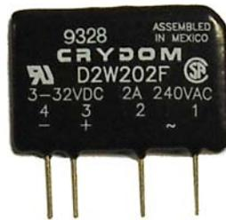
The only failure mode associated with these devices is the “half-wave” chattering problem. The only solution is to remove the old one and replace it with a new one. They were mounted in screw-type terminal blocks, so
