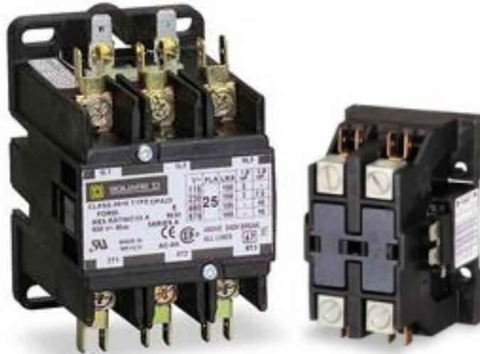
The large heating relays used in power controllers (or sometimes on-board the kiln itself) are known in the trade as “Definite Purpose Contactors” (or “DPC’s”). The smaller relay on the right can handle kilns rated up to 48-amps on single-phase 208-240vac power. The larger relay is used for all bigger kilns, and kilns wired for three-phase power.
